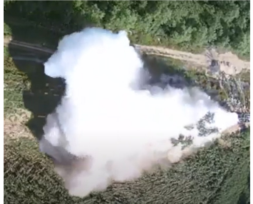
CO 2 pipeline rupture test by Dalian University of Technology in China. Source: https://www.youtube.com/watch?v=JC1bCIPbrsU
