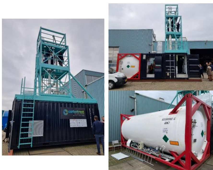
Figure 1. EverLoNG SBCC prototype pictures showing the CO 2 capture and liquefaction containers, as well as the liquid CO 2 storage tank.
